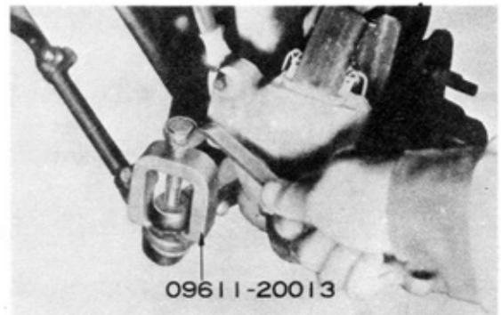
Fig. 7-37 Removing Tie Rod End
